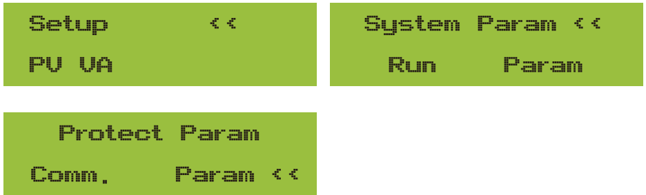
Pic 8.17 Submenus of the parameter setup
