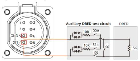
Figure 7-18 Wiring diagram for the DRM function
