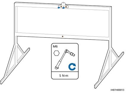
Figure 4-15 Secure the mounting bracket
