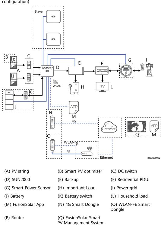
**Figure 2-3** Inverter cascading scenario (dashed boxes indicate optional configuration)
