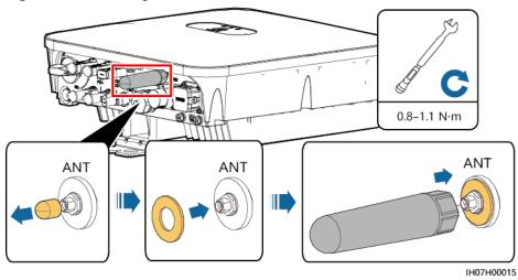
Figure 5-6 Installing a WLAN antenna
