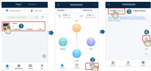
Figure 7-6 Uploading the physical layout template photo (App)
