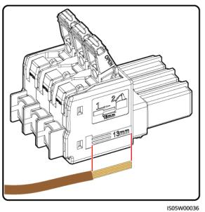
Figure 5-9 Length for cable stripping
