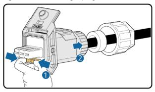
Figure 5-12 Removing a plug insert
