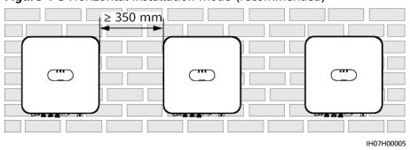
Figure 4-3 Horizontal installation mode (recommended)
