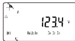
Voltage on A phase
