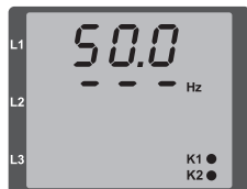
Fig. No rotation field direction detectable.
